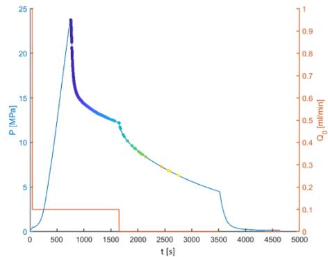
**Figure 3: Plot of pressure P (MPa) and Injection rate  $Q_0$  (ml/min) vs. time t (s) for GEMex03 experiment.**
