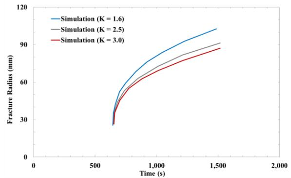
**Figure 7: Simulated fracture radius versus time for different fracture toughness.**
