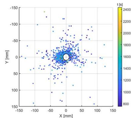
**Figure 5: Acoustic emission events for GEMex 03 projected onto the X-Y plane**
