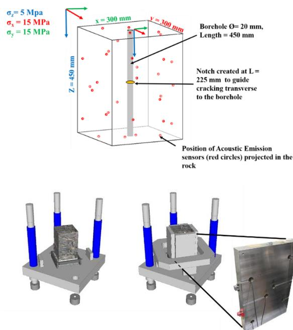
**Figure 1: Top: configuration of the acoustic sensors (red open circles) on the different sides of the samples, bottom: schematic of the triaxial press with the sample loaded on it; the slots for acoustic emission sensors are shown in the steel loading plates [3].**
