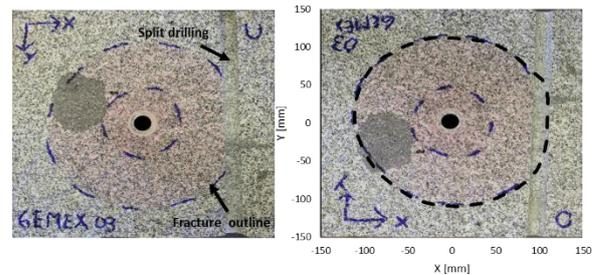
**Figure 4: Split plane with coloured fracture zone showing the fracture radius (GEMex03)**
