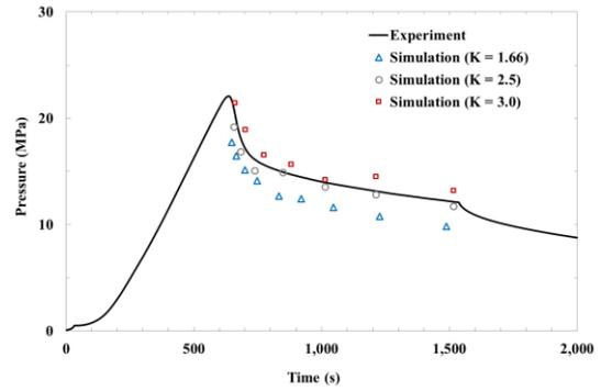
**Figure 6: Injection pressure versus time for different fracture toughness.**
